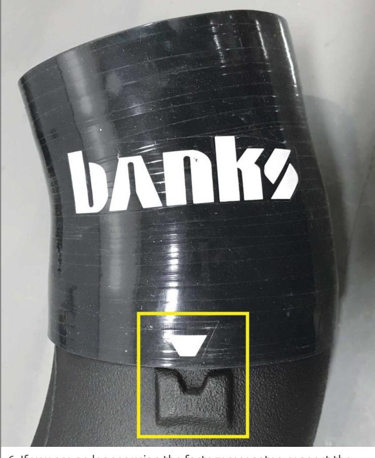
6. If you are no longer using the factory resonator, connect the intake tube elbow hose to the intake tube with the arrow
