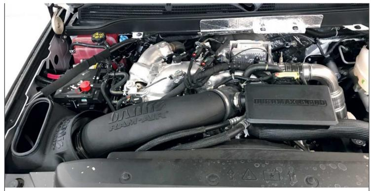
12. Re-connect the battery. Make sure to check all hose clamps for tightness and connectors for a sure fit. Make sure that the intake tube is not touching any engine components. You have successfully completed the installation!
