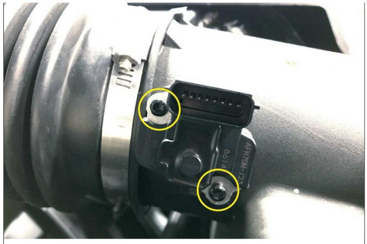
1. Disconnect the two screws securing the MAF sensor to the stock air box using a T20 Torx screwdriver, and remove the sensor.
