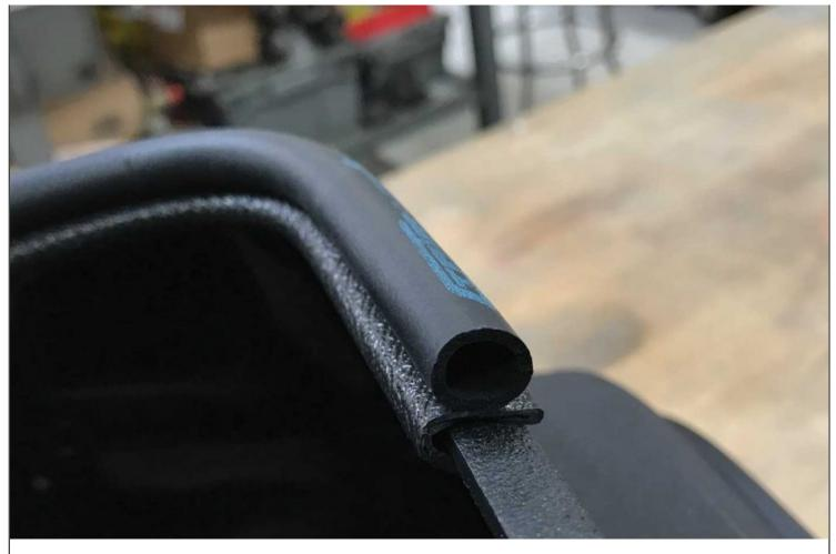
3. Prepare the Banks Intake Housing by installing the supplied seal pieces to the upper and side inlet openings. Trimming the trim pieces may be required for the best finish.
