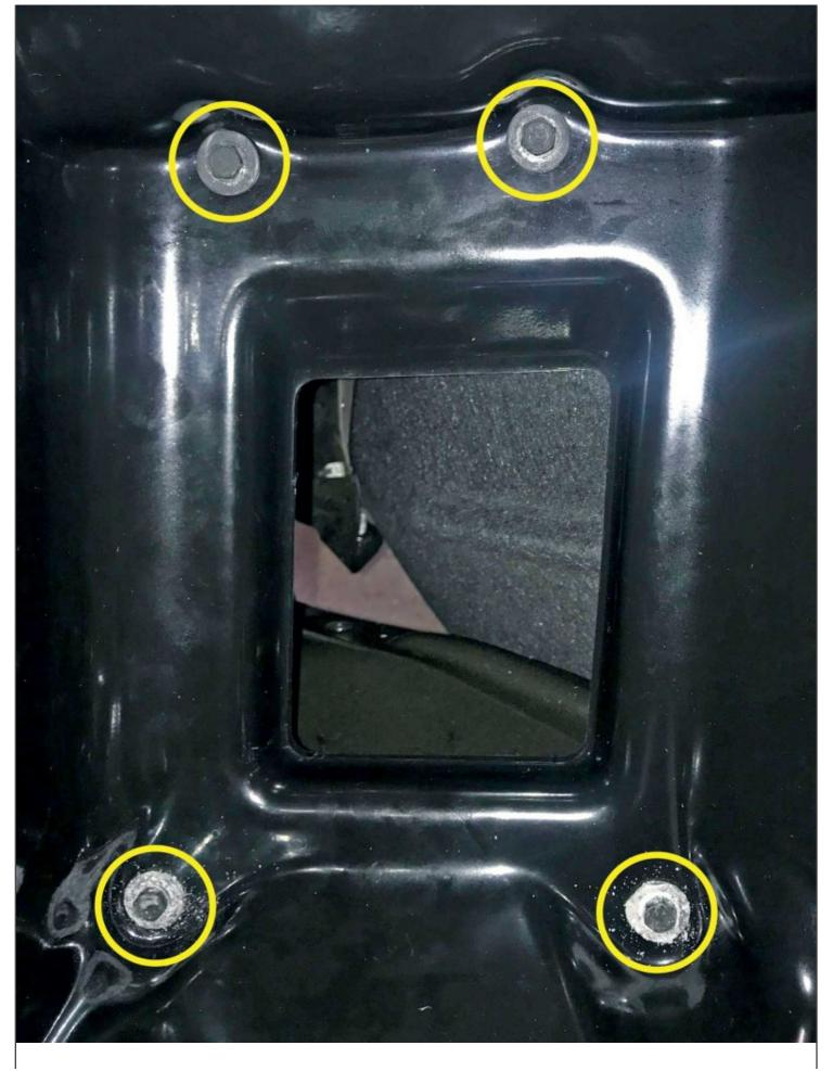
4. To install the Banks Intake Housing, secure the box with the outlet facing the center of the vehicle and bolt using the stock tray's previously removed bolts.
